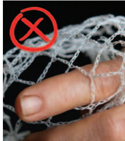
This is the wrong type of netting - you can easily poke your finger through. It fails the 'finger test'.
